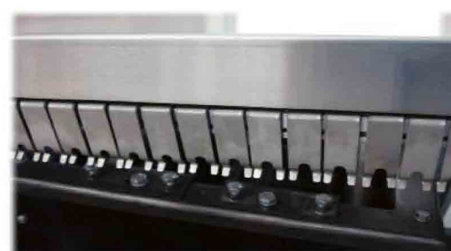
Finger conveyor for pallet or pallet-less operation.
