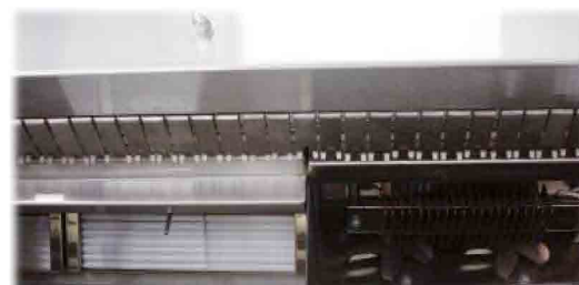
Independently controlled infrared and forced air convection preheaters compatible with VOC-free fluxes.
