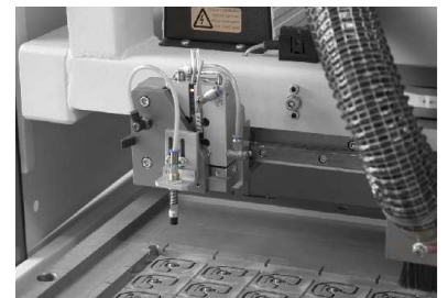
Automated faulty part removal gripper or suction unit respectively
