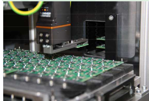
Automated Printed circuit board feeding with cutting unit removal into tray
