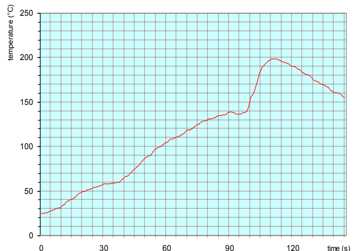
T^\circ measured on the topside of the PCB on a lead-free soldering machine.
