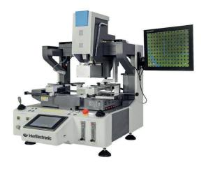
4V-groove PCB support, rapid positioning, convenience, accuracy, can fit for all kinds of PCB board. Flexible and removable universal fixture has protective effects and no damage to the PCB board, suitable for all kinds of BGA repair.
