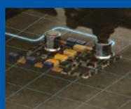
Auto Adaptive Sequencing defines placement priorities and rules to avoid collision. It takes into account component and nozzle shapes, characteristics of the PCB and the trajectory of the heads.
