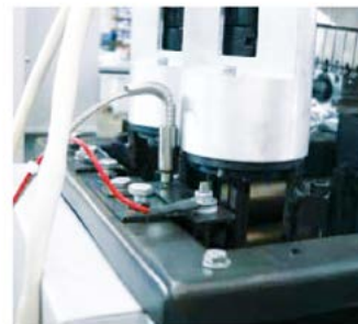
Solder level sensor with alarm
