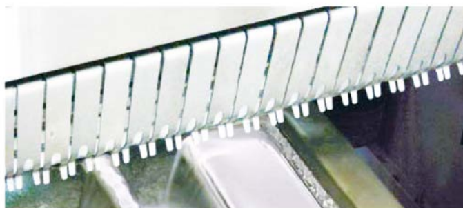
Dual Wave Option shown above - turbulent wave for SMD (optional) and laminar wave for through-hole soldering.
