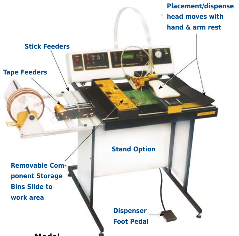
Model MPP-21 Benchtop pick & place with dispenser, feeder rack, tape & stick feeders, and stand option
