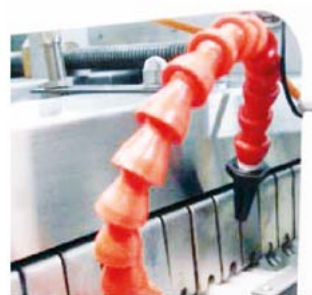
Recirculating finger cleaner option with spray spout and brushes
