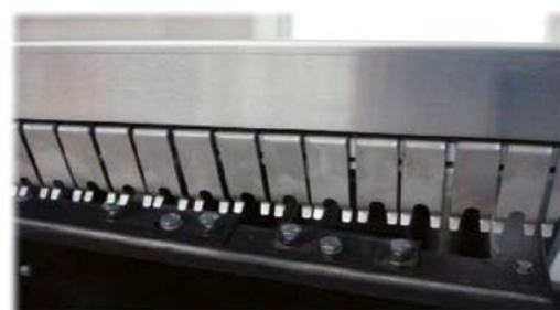
Finger conveyor for pallet or pallet-less operation.
