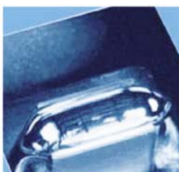
Solder wave for 14-20 pin IC shown (WN-10 nozzle)
